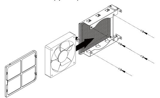
First remove the internal accessories in the chassis, position the fan expansion cage from the inside, then secure with the included 4pcs screws.
