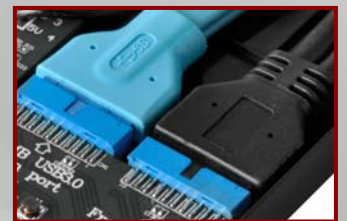
Unique USB 3.0 19pin daisy-chain design retains Mini-ITX chassis' original USB port function
