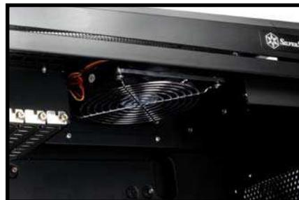
Top exhausting 120mm fan assist RV02-E's stack effect cooling.
