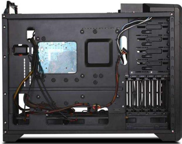
SilverStone has implemented various openings and cable tie down bridges around the motherboard to assist users in routing cables. This design not only enhances the aesthetics of component installation, but also ensures unimpeded airflow in the chassis.
