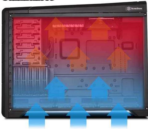
Making a debut for the first time in a tower chassis, SilverStone's own "Air Penetrator" 180mm fans are included in the RV02-E for improved air intake efficiency and flexibility.
