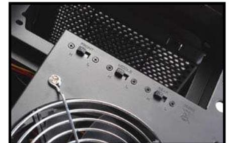
Three 180mm fans can be adjusted independently to run at 700rpm or 1200rpm.
